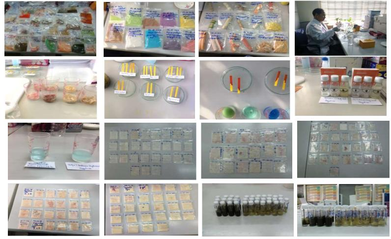
Test kit analysis to Borax, Formalin, Sodium Hydrosulfite, Coliform in food, water & ice and Cleanliness
