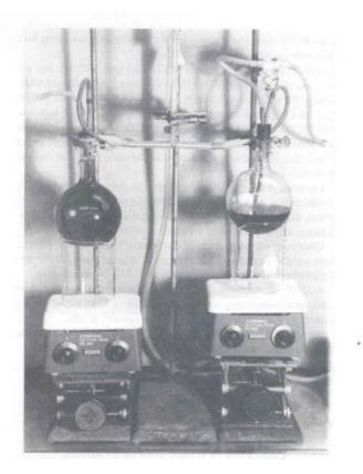
Reflux Apparatus (Solvent saver apparatus)
